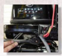
Mount the standard bracket to your motor. NOTE: our bracket is designed to fit as many motor models as possible. You may need to adjust how you mount it to make it fit your motor. Just remember to keep the linkage mounting point as close to the center of the motor as possible.
