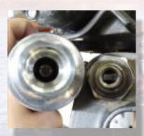
Line up the slot in the motor shaft with the shaft inside the coupler on the actuator.
