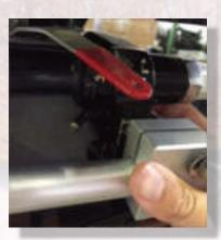
Place the hook arms of your bracket around your motor's clamps and position the blocks flat against the clamps.
