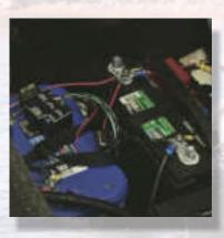
Connect the Red (+) wire from the relay control box to the Red (+) post on your battery, then connect the Black (-) wire from the relay control box to the Black (-) battery post.
