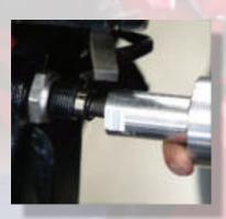
Slide the motor onto the coupler making sure that the shafts engage one another.
