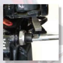
Once you have determined which side the linkage will be mounted on, you can insert the actuator through the steer tube. The threaded eyelet of the actuator will need to be inserted into the steer tube first and will need to end up on whichever side of the motor the linkage will be mounted on. NOTE: You will need to remove the grey wiper nut from the actuator before inserting it. Once the actuator is in place, tighten the wiper nut onto the end of the steer tube nearest the actuator eyelet.
