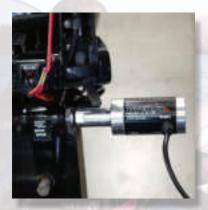
The wavy washer will now allow up to 1/4" extra turn so you can position the wires coming straight forward into the boat. Use your adjustable wrench to tighten the motor in place.
