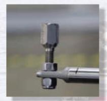
Remove the nylock nut from the bottom of the standoff bolt assembly and twist the standoff bolt into the threaded eyelet on the actuator. Then reinstall the nylock nut.
