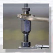
Remove the top bolt from the standoff bolt. Place the plastic washer in between the bronze bushing on the linkage arm and the standoff bolt. Then replace the top bolt so that it goes through the bronze bushing and plastic washer before tightening into the standoff bolt. Use a 3/16" Allen Wrench to tighten.
