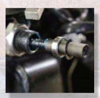
Place the included wavy washer from the motor packaging onto the actuator coupler. NOTE: The wavy washer will allow you to position the motor wires properly in STEP 10 so it is very important you do not skip this step!
