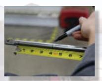
Using your permanent marker, mark the spot on the actuator that is exactly halfway between the wiper nut and the mark you made in step 16.
