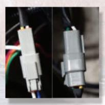
Connect the two-button switch to the relay control box making sure to line up the locking connections on the gray connectors. Then connect the motor to the relay control box, again lining up the locking connections.
