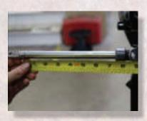
Now, using your control, extend the actuator out as far as it will go. Using a tape measure, measure the distance between the wiper nut and the mark you made in Step 16.
