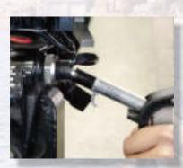
Clean the Steer Tube of debris–a few shots from an air compressor should do the trick.
