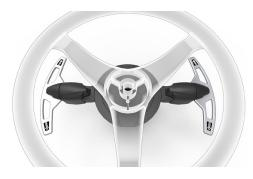
Every MAGNUM and MAGNUM MAX Jack Plate comes standard with a two-button switch control. Our wheelmounted Paddle Switch is an optional upgrade which allows you to keep your hands on the wheel and operate your Jack Plate.
