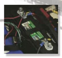
Connect the Relay Control Box to the battery. The Red (+) wire will go to the Red (+) battery post and the Black (-) wire will go to the Black (-) post
