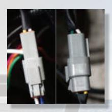
Mount your Two-Button Switch wherever you would like it and route the switch cable back to the control box. Connect the switch cable and the motor cable to the control box. Ensure that you line up the locking mechanisms of each connector and that they fully lock together.
